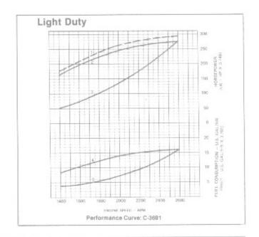
Curves shown above represent engine performance capabilities obtained and corrected in accordance with SAE J1349 conditions of 29.62 in. Hg (100 kPa) barometric pressure [300 ft. (90 m) altitude], 77° F (25° C) inlet air temperature, and 0.30 in. Hg (1 kPa) water vapor pressure with No. 2 diesel fuel.
